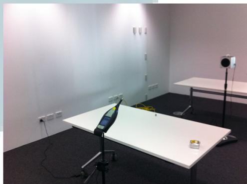
Figure 3. Measurement of background noise and pink noise
